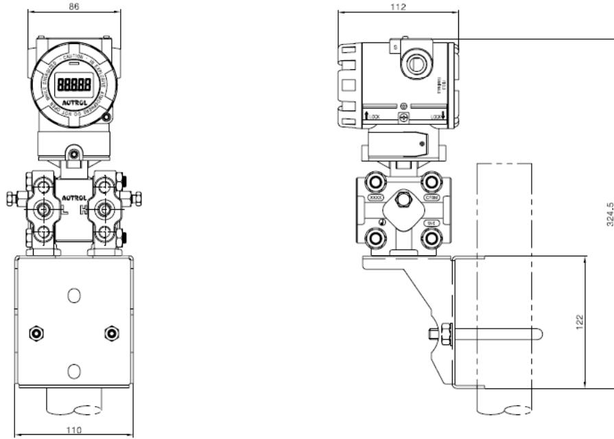
2" Pipe Mounting Bracket Model Flat Type
