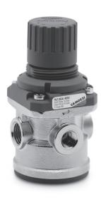
Series N pressure regulators are available with G1/4 and G1/8 ports. Their design incorporates a self relieving diaphragm so as to allow decremental adjustments.
