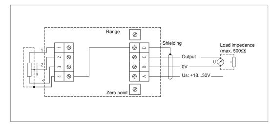
The output signal rises when the wiper is moved from position 1 to 3 (see connection diagram in the corresponding data sheet). For the reverse function, simply switch the connections 1 and 3 in the MUK housing.
