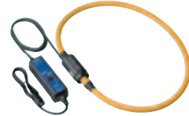
FLEXIBLE CLAMP ON SENSOR CT9667 500A AC/ 5000A AC (selectable), φ254mm(10"), Power supply: LR06 alkaline battery or AC ADAPTER 9445-02/03 (sold separately)
