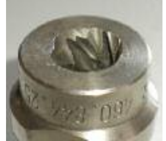
Fig. 2: Wear of a full cone nozzle
