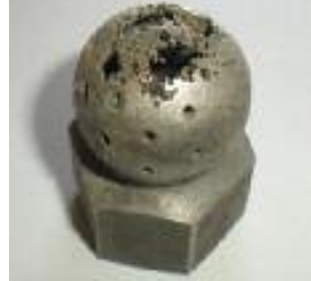
Fig. 1: Chemical corrosion of a spray ball
