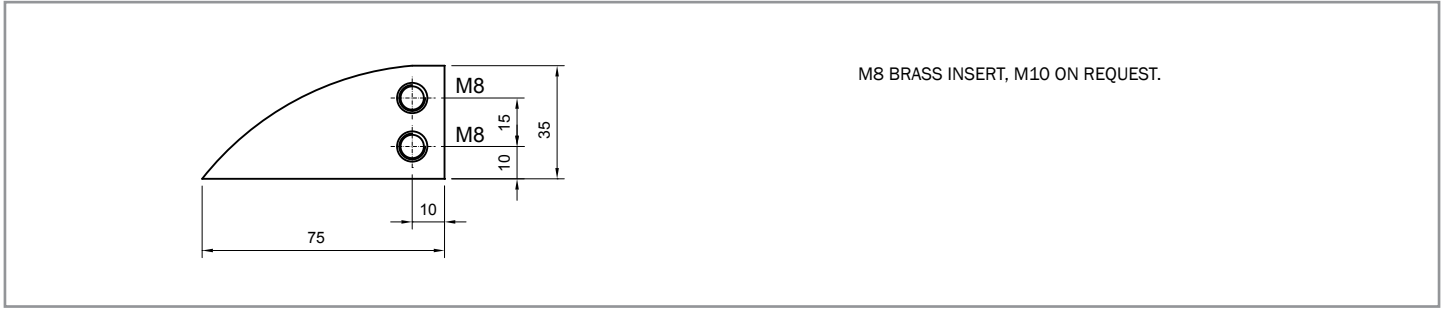
M8 brass insert, M10 on request.
