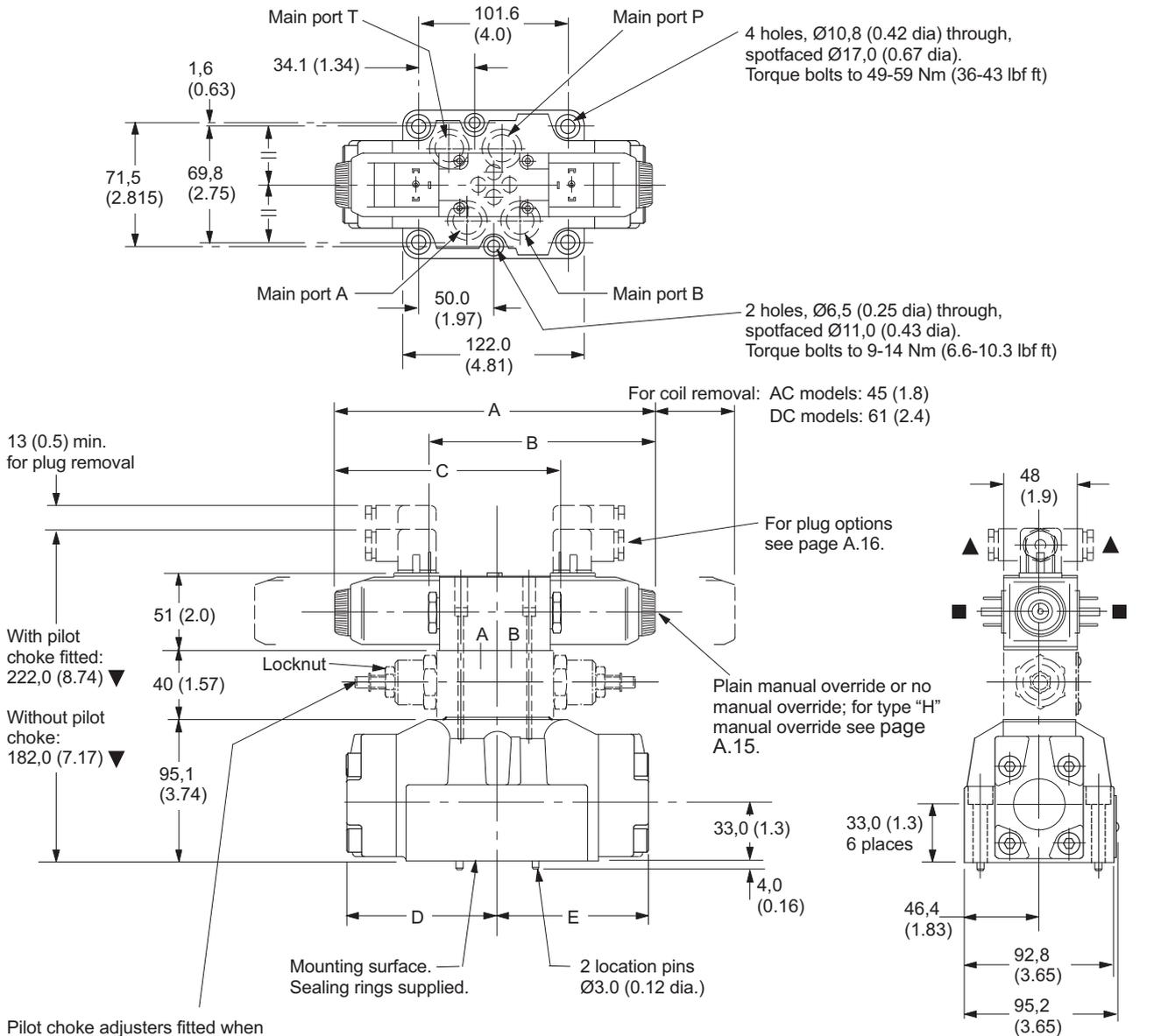
Pilot choke adjusters fitted when Model Code [4] = 2, 3, 27 or 28. To adjust, turn locknut counter-clockwise, then turn screw clockwise to slow down rate of spool travel, or counter-clockwise to increase the rate. Retighten locknut to 25-30 Nm (18-22 lbf ft).
