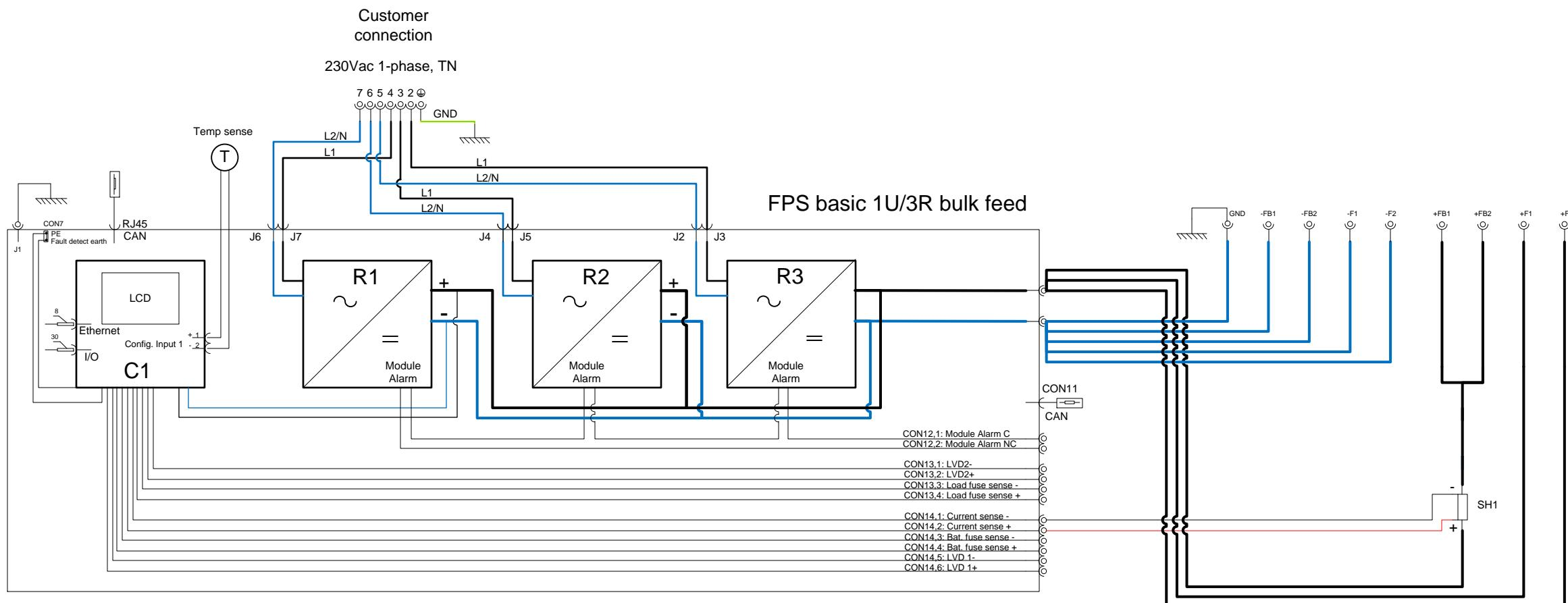
The Schematic/Connection Drawing shows the position of the relay contacts when the Power System is in its alarm mode of operation (relay coils are then de-energized). The relay outputs are preprogrammed from factory (Factory Settings).
