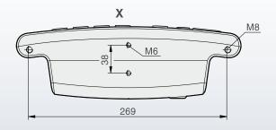
mm tolerances ISO 8015 ISO 2768 - m H < 6 mm: ±0.2 mm
